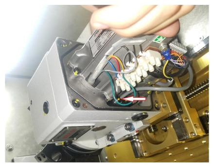
• Remove the ratchet wrench and release the emergency button. Set the machine to handle or jog mode and use the operator panel to move the turret clockwise and counterclockwise a few times to confirm the problem is fixed. Press the emergency button once again to mount the back cover on.
