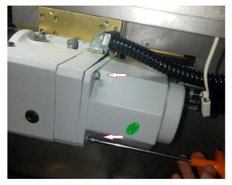
• Remove four screws, one on each corner of the turret's back cover with a 5mm hex wrench.
