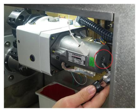
• Continue turning the turret until the yellow light on the bottom turns on.
